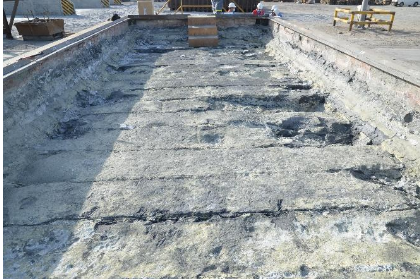
Figure 2. Autopsy of a copper insert cell with graphitized cathode block, 976 days old.
