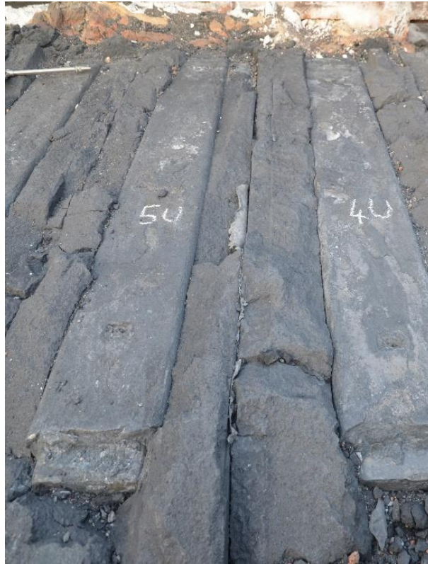
Figure 4. trace of liquid aluminium metal observed on collector bars.
